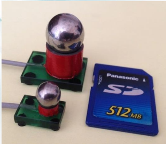
Test examples of reaction sphere with cylinder piezoelectric transducer
